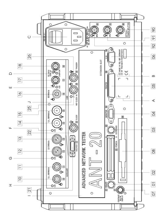
Fig. O-2 ANT-20 connector panel
