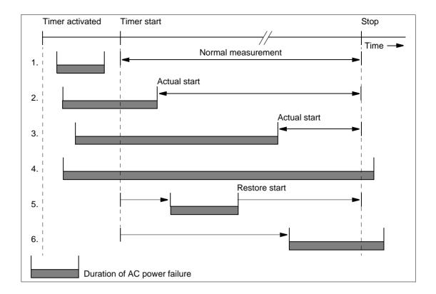
Fig. O-43 Examples of ANT-20/ANT-20E behavior in the event of an AC power failure (timer-controlled measurements)
