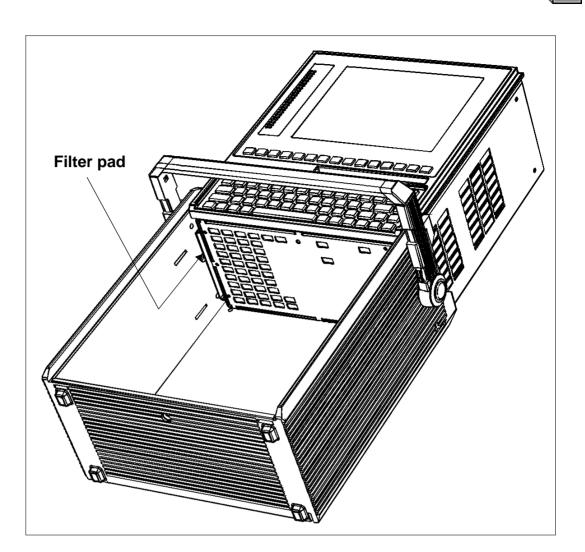
Fig. M-4 Replacing the ANT-20 filter pad
