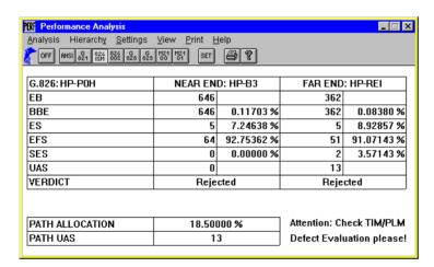
Fig. VI-36 "Performance Analysis" window showing ITU-T G.826 ISM (in-service measurement)
