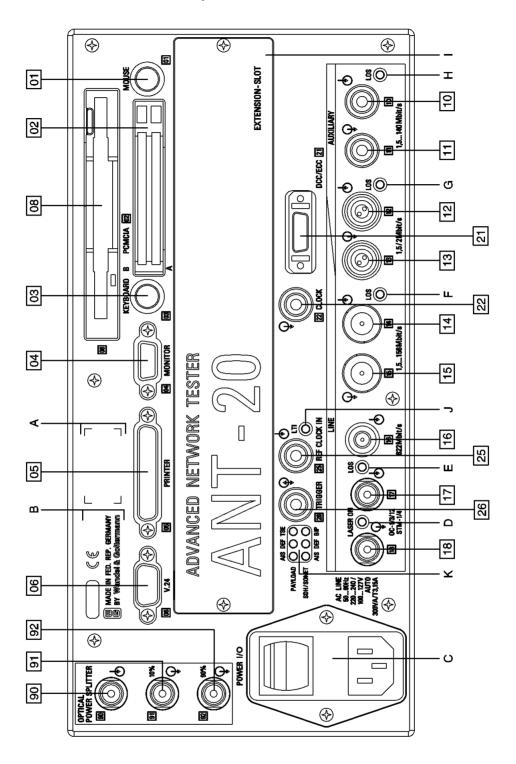
Fig. O-4 DominoCOM ANT-20 connector panel
