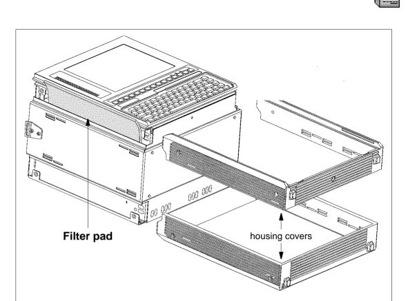
Fig. M-6 Replacing the ANT-20E filter pad
