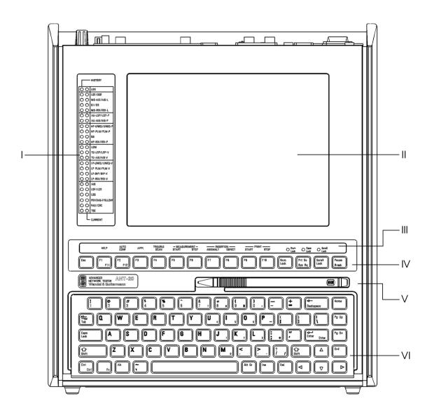
Fig. O-1 ANT-20, ANT-20E front panel
