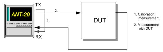
Fig. A-62 Jitter transfer function measurements setup
