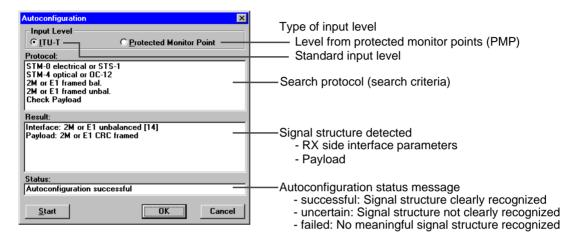
Fig. VI-5 "Autoconfiguration" dialog
