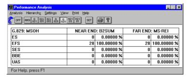
Fig. VI-38 "Performance Analysis" window showing an ITU-T G.829 analysis
