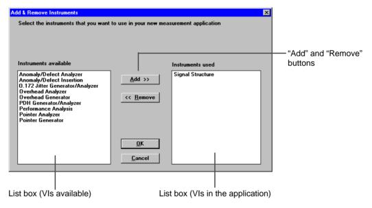
Fig. O-17 The "Add & Remove Instruments" dialog window of the Application Manager
