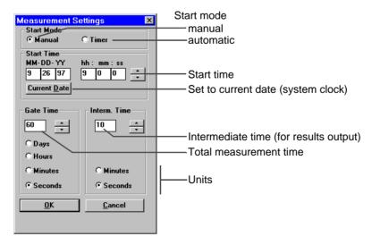
Fig. O-25 The "Measurement Settings" dialog window
