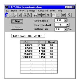
Fig. A-61 Fast MTJ measurements window
