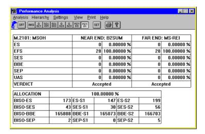
Fig. VI-40 "Performance Analysis" window showing an ITU-T M.2101 analysis
