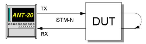
Fig. A-50 DCC/ECC bit error test setup
