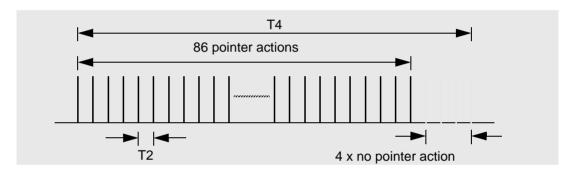
Fig. TB-10 "86-4" sequence with missing pointer
