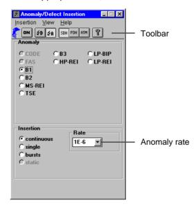
Fig. O-26 The "Anomaly/Defect Insertion" window
