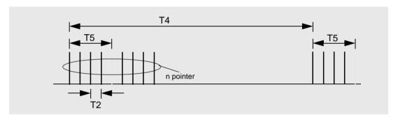
Fig. TB-7 Pointer burst with missing pointers
