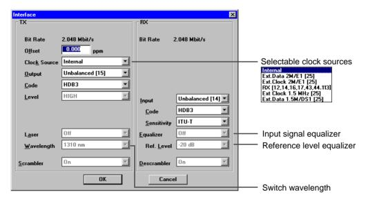
Fig. VI-3 "Interface" dialog with "Clock Source" list box
