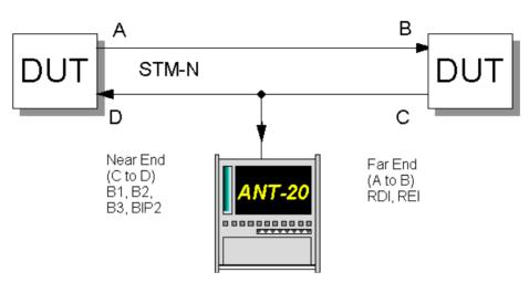
Fig. A-34 In-service monitoring setup
