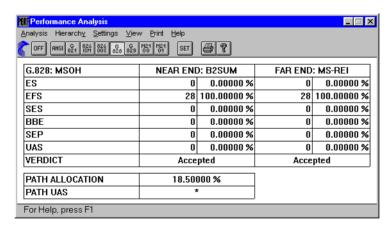
Fig. VI-37 "Performance Analysis" window showing an ITU-T G.828 analysis
