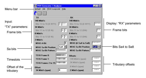
Fig. VI-31 Elements of the "PDH Generator/Analyzer" main window
