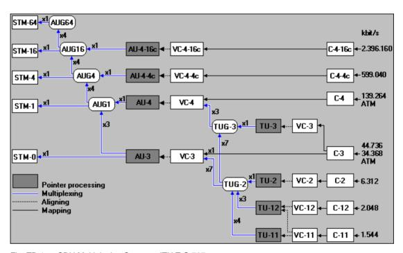
Fig. TB-1 SDH Multiplexing Structure ITU-T G.707
