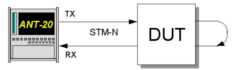
Fig. A-27 Bit error rate test setup
