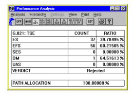
Fig. VI-35 "Performance Analysis" window showing ITU-T G.821 analysis
