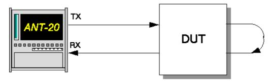
Fig. A-58 Fast MTJ measurements setup
