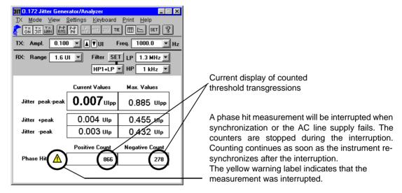
Fig. A-72 Phase hit measurement
