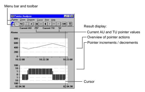
Fig. VI-27 Elements of the "Pointer Analyzer" main window
