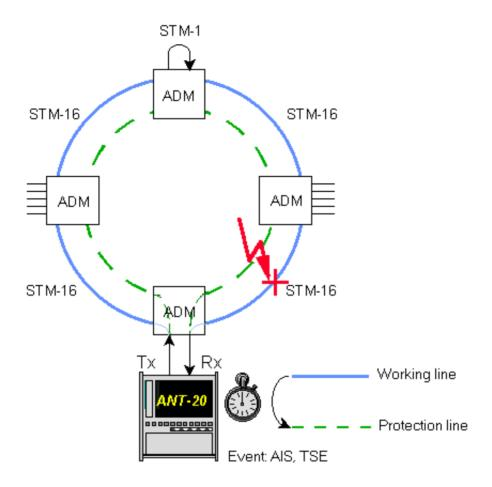
Fig. A-24 APS switching time setup
