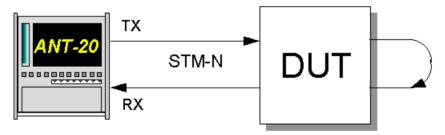
Fig. A-35 Out of service measurement setup
