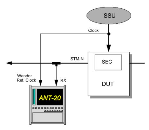
Fig. A-79 Wander measurements setup
