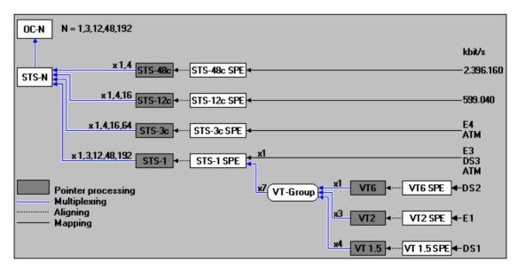
Fig. TB-2 SONET Multiplexing Structure ANSI T1.105-1995
