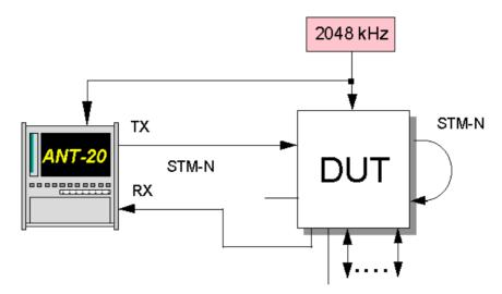
Fig. A-38 Pointer stress test setup
