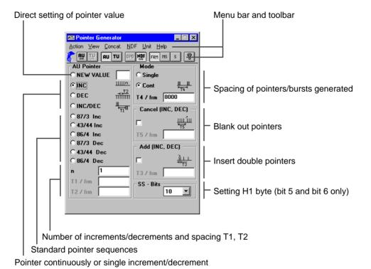
Fig. VI-25 Elements of the "Pointer Generator" main window
