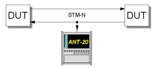
Fig. A-10 In-service monitoring setup
