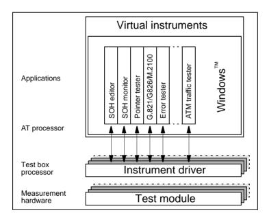
Fig. I-3 ANT-20 software architecture
